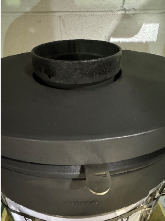
Air control Maximum setting
